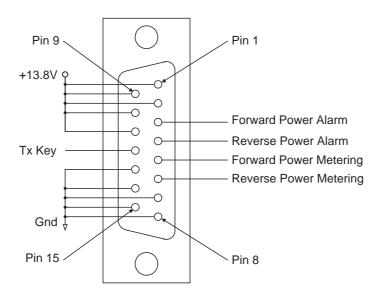
Figure 2.5 T858/859 D-Range Wiring - Rear View
